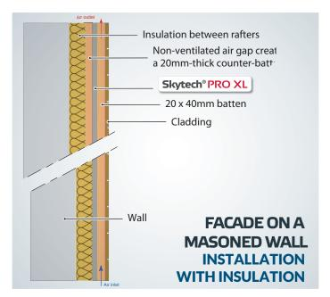
In direct contact or with a non-ventilated air gap : SKYTECH PRO XL allows to cover the thermal bridges at rafters thus avoiding the cross-installation of an external additional insulation.
